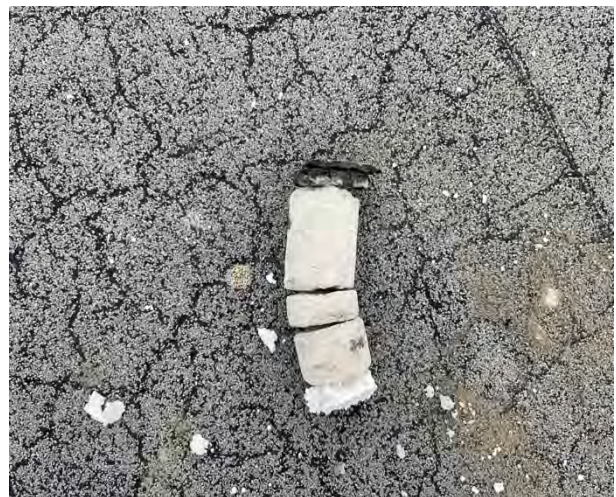
We did a core on the roof and determined the roofing assembly consists of a concrete roof deck, 1" Styrofoam insulation, 5" light weight concrete, and a solidly attached 4-ply built up roof.
